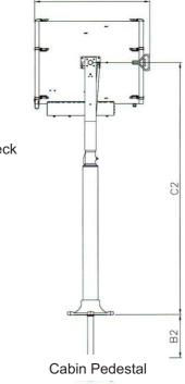
3 holes  $\emptyset$ 11.0 on a 174.0 PCD. Central hole  $\emptyset$ 52.0
